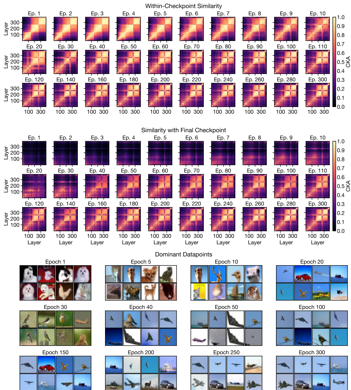
Figure F.1: Fine-grained analysis of the evolution of the block structure in a ResNet-110 (1x) model. This plot shows the evolution of block structure for the same network as in Figure 8, but with greater temporal granularity. As in Figure 8, we find that the shape of the block structure is defined early in training (top row). However, comparing these different model checkpoints to the final, fully-trained model reveals that the block structure representations at different epochs are considerably dissimilar, especially during the first half of the training process (middle row). The corresponding dominant datapoints also vary over training, even after the block structure is clearly visible in the within-checkpoint similarity heatmaps (bottom row).
