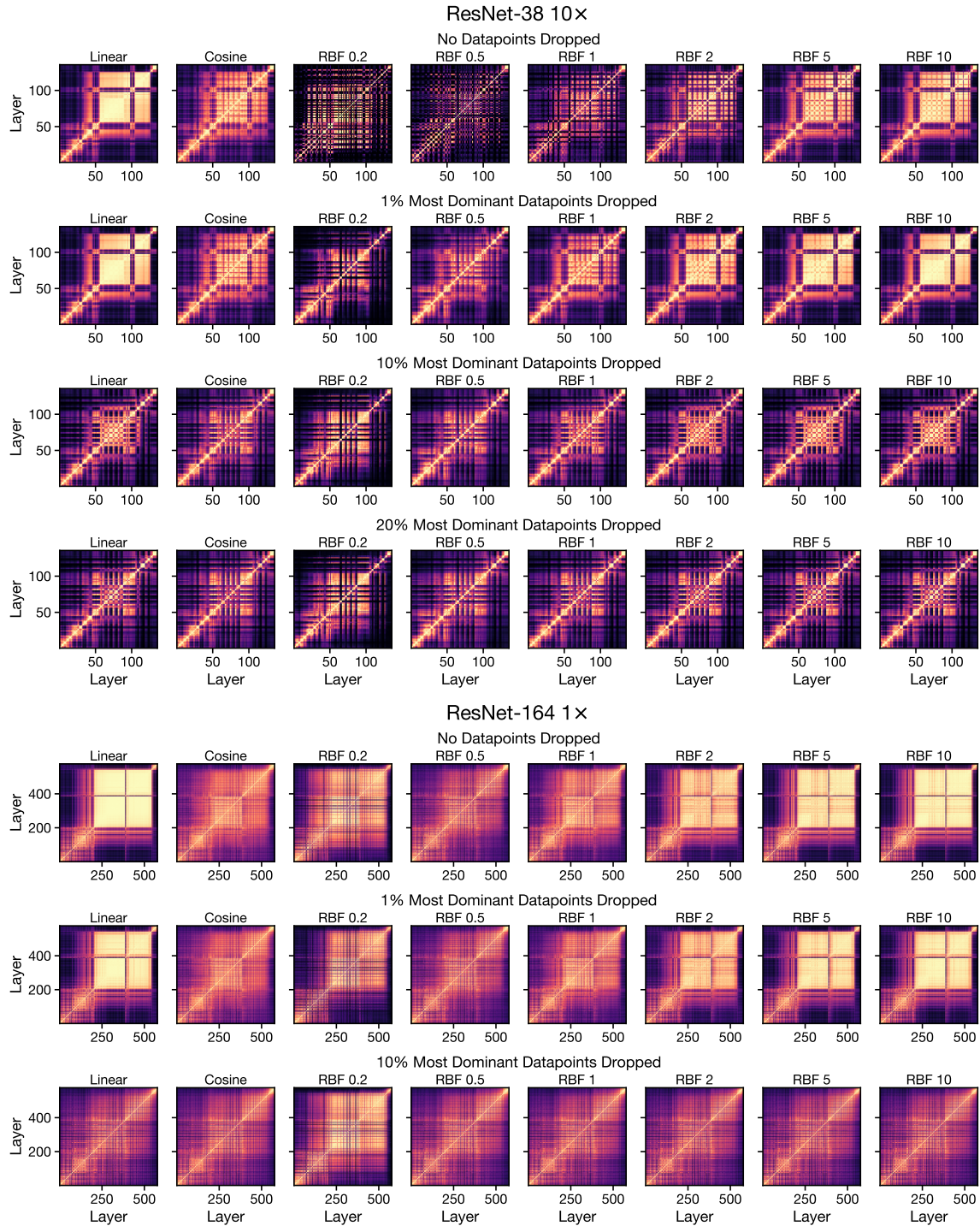
Figure J.3: Removing dominant datapoints eliminates both blocks and differences among kernels in CKA representational similarity heatmaps. We remove the top k\% of examples according to the magnitudes of their projections on the first PC in layer 76 for ResNet-38 10\times and layer 276 for ResNet-164 1\times . Because 14/128 datapoints are dominant in the minibatch kernel matrix shown in Figure J.2, we provide results for removing 20% of datapoints for that network, although they look only modestly different from the results obtained by removing 10% of datapoints.
